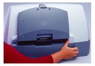
4. Remove the scanner front panel.
